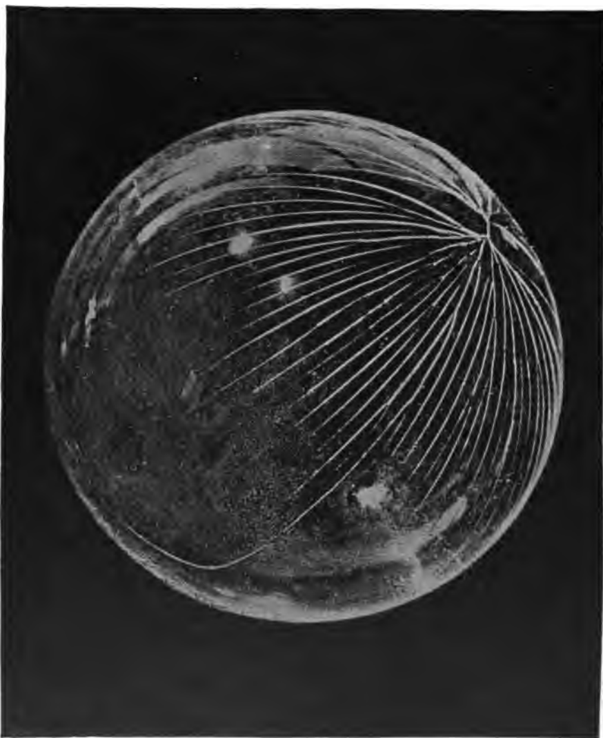
FIG. 67. — GLASS GLOBE, CRACKED.
